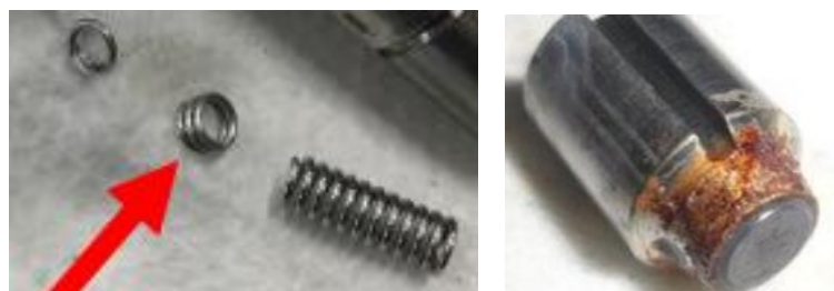
Figure 16. Broken spring (left) and corroded plunger (right).
